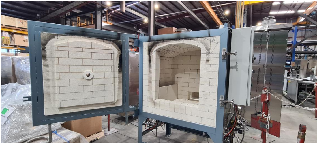
Open kiln door more than 90° angle
