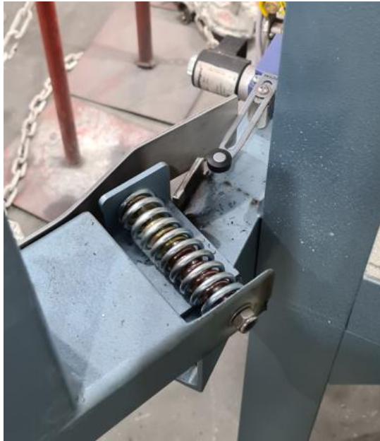
Purge limit switch
